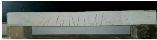
Fig 2: Typical crack pattern of the flexural beam
