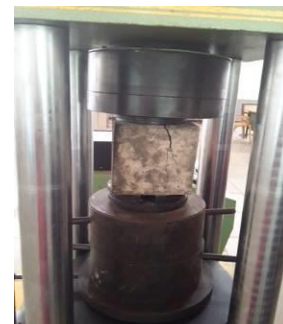
Fig.3.Test setup for compressive strength
