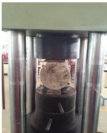
Fig.7.Test setup for split tensile strength of cylinder
