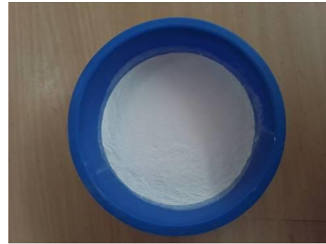
Fig.1.Egg shell powder sieved through 90 micron sieve
