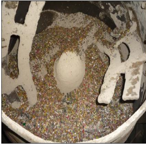
Fig. 2 Dry mix of geopolymer contents with metalized plastic waste fibers
