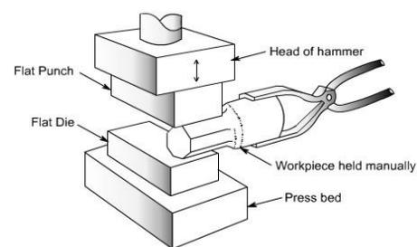
Fig. 1 Open die forging process [NPTEL notes]
