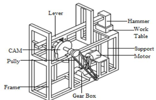
Fig. 3 3D View of automatic forging model
