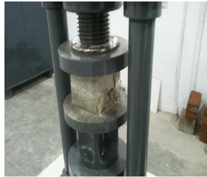
Fig 2.3 compression test for concrete cube
