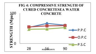
From the test results ,it has been observed that the compressive strength of blended cement concrete marginally better than conventional cement concrete .This may be attributed to the secondary hydration reaction in the case of blended cement concrete leading to long term in strength. The results of resistance of concrete to sea water attack are reported in table. From the table it is evident that there is a loss in weight in any type of concrete resulting in the deterioration of concrete.
