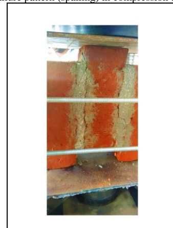
Fig. 9. Failure pattern in shear bond test specimen
