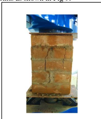
Fig. 7. Failure pattern (cracking) in compression test specimen
