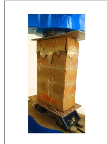
Fig. 8. Failure pattern (spalling) in compression test specimen
