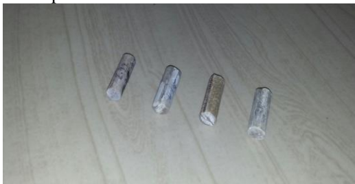
Fig 5: Wear Test Specimens of different compositions
