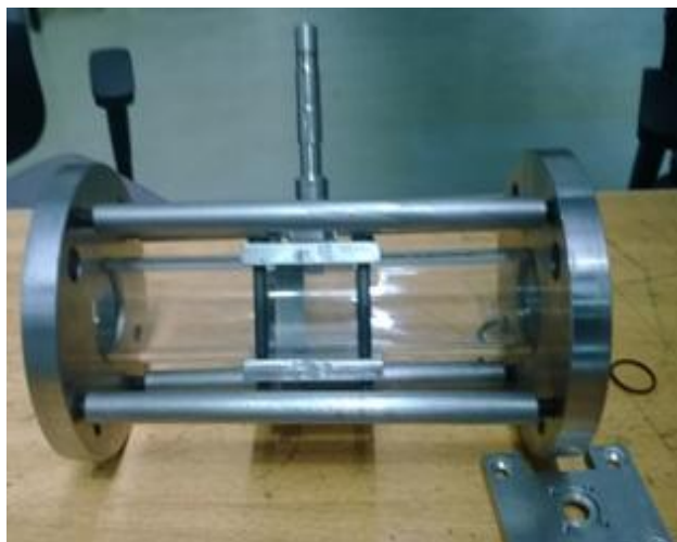
Fig.3. Vortex flow meters with trapezoidal shape bluff body
