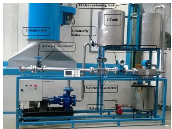
Fig. 2. Test facility for flow visualization Experiments
