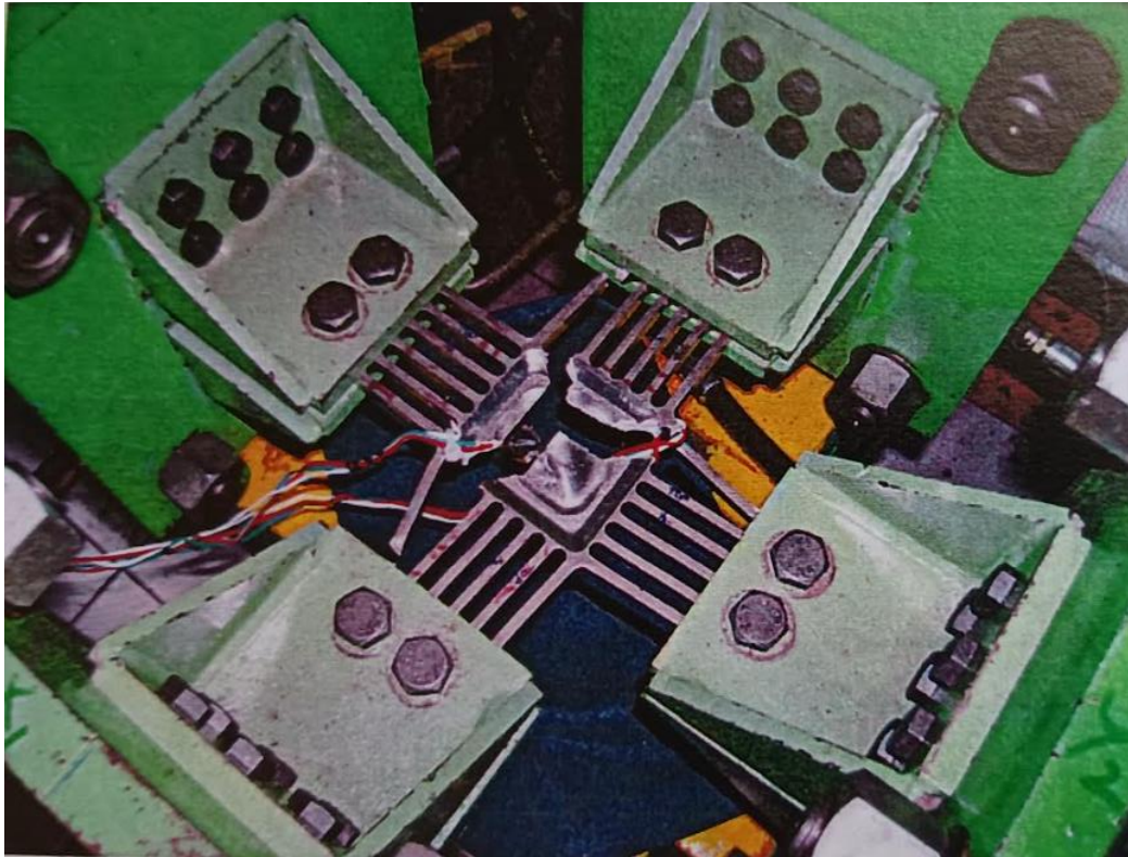
Figure 11: Solution Treated & Aged (STA) Ti-6Al-4V specimen under equi-biaxial loading
