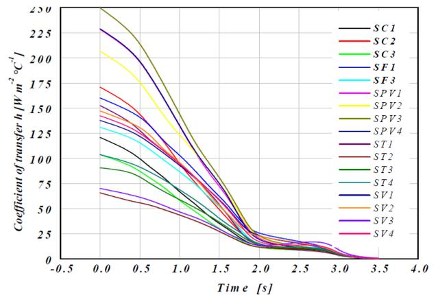
Fig.5. Variation of heat transfer coefficient (h) of various surfaces for a ventilated disc in transient case
