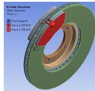
**Fig.8. Boundary conditions and loading imposed on the disc-pads**
