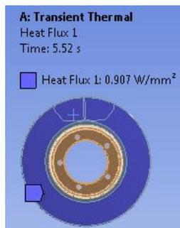
Fig.1. Application of Heat flux
