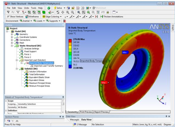
**Fig.7. Thermal load imported in structural analysis.**
