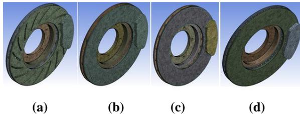
Fig.3. Meshing of the disc
