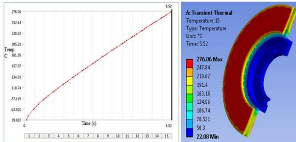
**Fig.6. Temperature distribution of a various ventilation disc**
