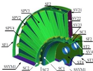
Fig.4. Various surfaces for a ventilated disc
