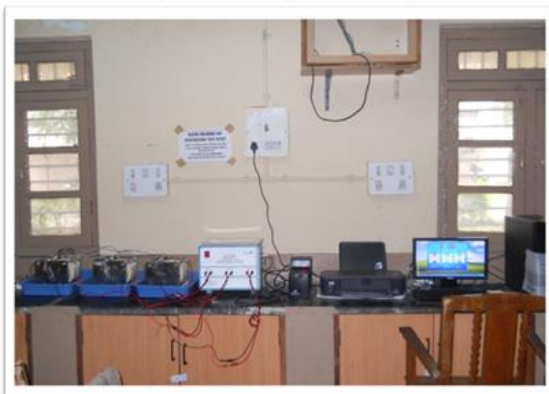
Fig 3.2 Laboratory Setup of RCPT.
