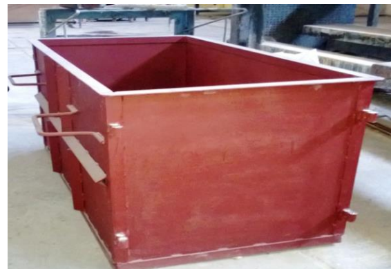
Fig 3. Test tank used for Lateral Loading
