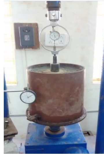
Fig 2. Setup used for Axial Loading
