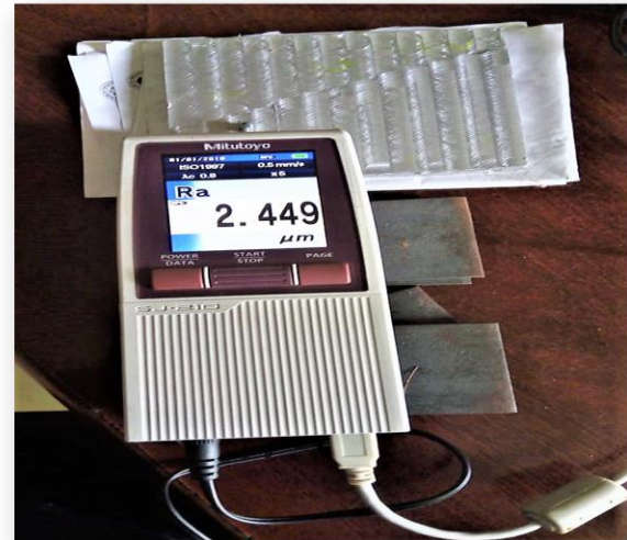
Fig.1 mean value (Ra) measured by in micrometres set up
