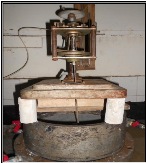
FIG. 1 VANE SHEAR APPARATUS WITH SOIL SAMPLE
