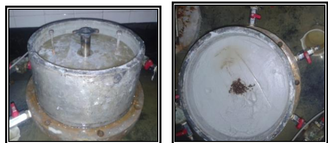
FIG. 2 INSTALLATION OF VERTICAL DRAIN
