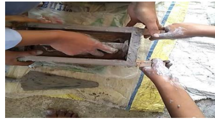
Fig 12 Brick removed from mould
