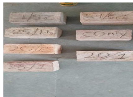
Fig 4.21 Brick after burned kiln
