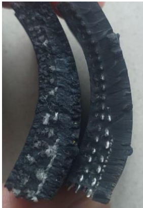
Fig 1.3- Left-Physically treated rubber with sharp object, Right-Non treated sample
