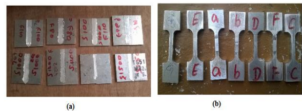
Fig. 3. Welded Joints and Tensile Specimens
