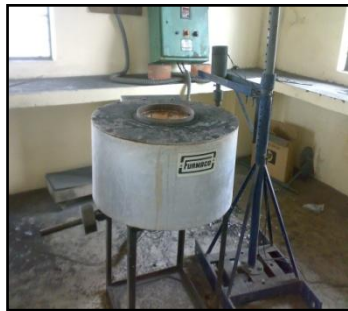
Figure 4.1: Al 2219 melting in the electrical resistance furnace.
