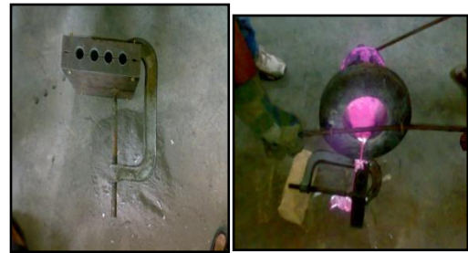
Figure 4.6 ASTM Casting Dies. Figure 4.7: Hot liquid molten metal is poured in ASTM Dies.
