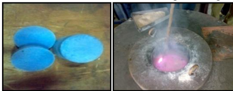
Figure 4.2: Degassifier Hexachloro ethane Figure 4.3: Degassifier is mixed in crucible.
