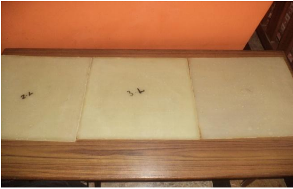
Fig 5: Prepared laminates of neat matrix, 2L and 3L WSM reinforced epoxy/glass sample after post curing.
