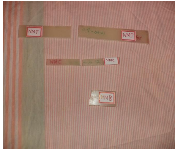
Fig 23 : Epoxy/glass samples of neat matrix(NM) after all mechanical tests.
