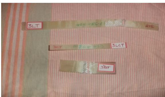
Fig 22 : Epoxy/glass samples of 3L WSM mat after all mechanical tests.
