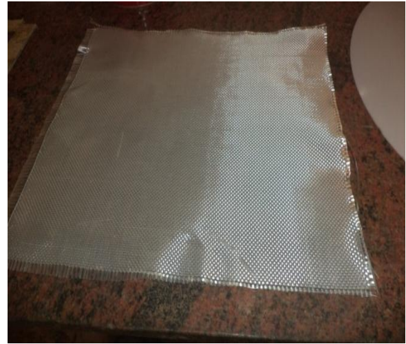
Fig 2: WSM Glass fibre 300*300*4(mm).
