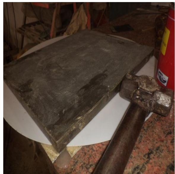
Fig 4: Load is kept to remove excess of resin.
