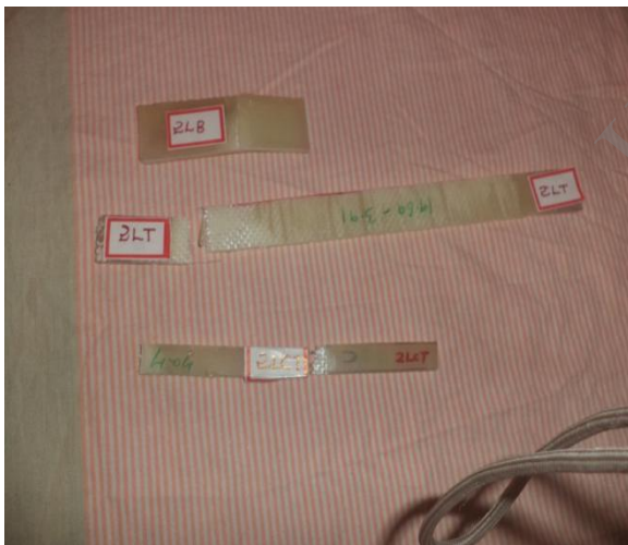
Fig 21 : Epoxy/glass samples of 2L WSM mat after all mechanical tests.
