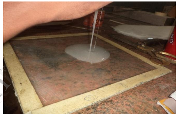
Fig 3: Resin is added to prepared mould.
