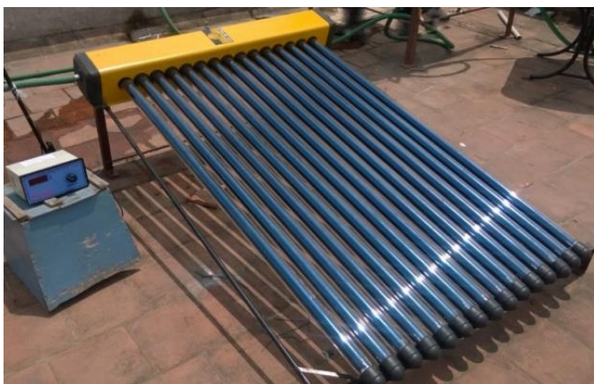
Fig. 1: Evacuated tube solar water heater
