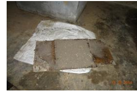
Fig. 6. Compacting in a mould before keeping into hot press.
