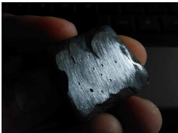
Fig No. 2 Surface Grounded Sample showing indentation after Rockwell test
