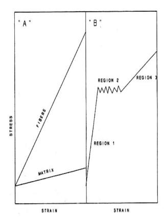
Concrete, reinforced with fiberglass, has been found to perform very well. On the stress/strain chart (Figure 3, left side "A") shows each component (cement matrix and glass fibers) by themselves. (Figure 3, left side "B") shows the composite system.
