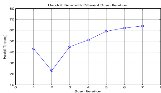
Fig. 3. Handoff time with different scan iteration
