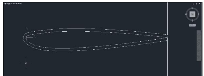
Figure 4 - NACA 23012-airfoil profile visualized in AutoCAD 2013
