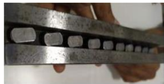
Fig. 1.2 Experimental set-up for HE testing
