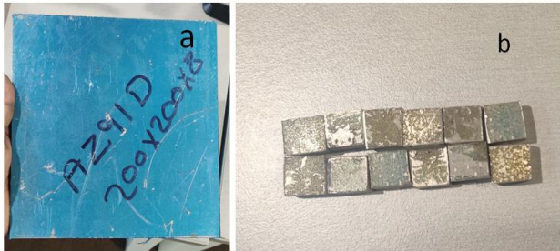
Figure - 3.1 a) AZ 91D plate b) AZ91D Specimen
