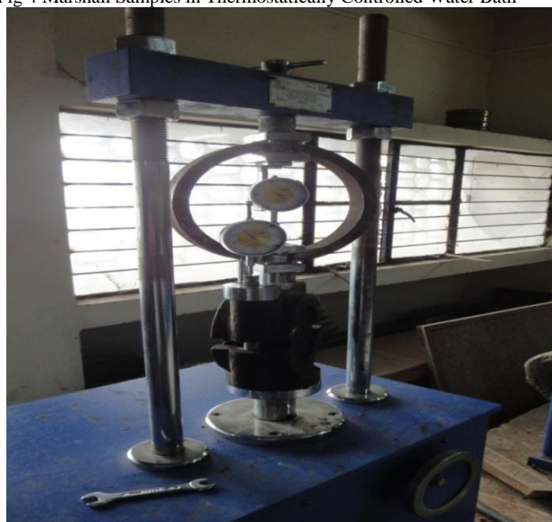
Fig 5 Marshall stability test
