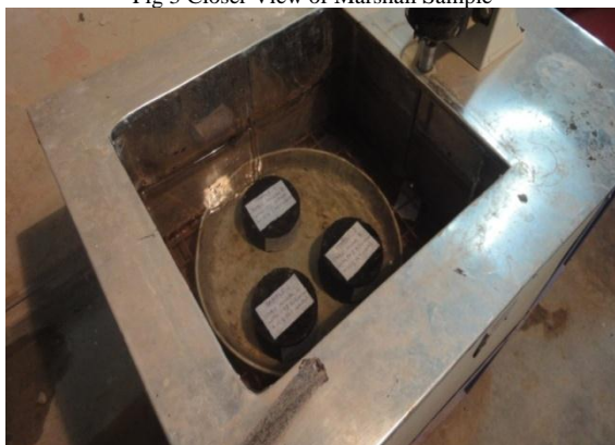
Fig 4 Marshall Samples in Thermostatically Controlled Water Bath
