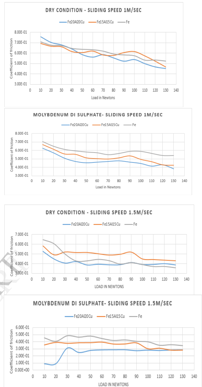
Figure 4. Variation of coefficient of friction at incremental load for various lubricants and sliding speeds.
