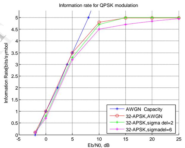
Fig.4. Information rate for a 32-APSK modulation
