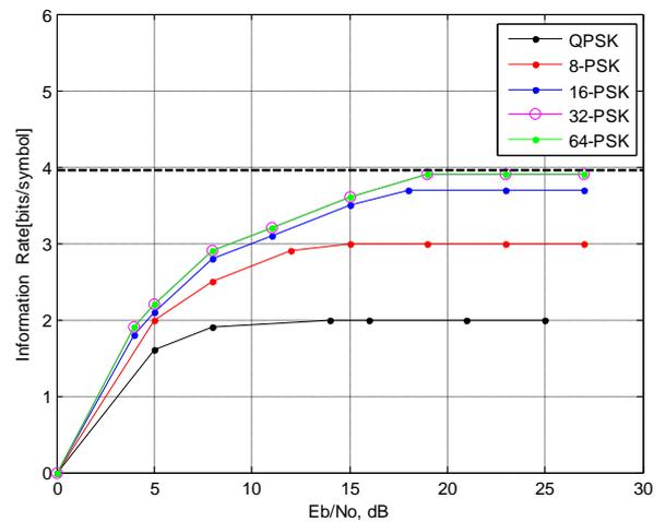
Fig.3. Upper bound of Information rate for an M-PSK modulation
