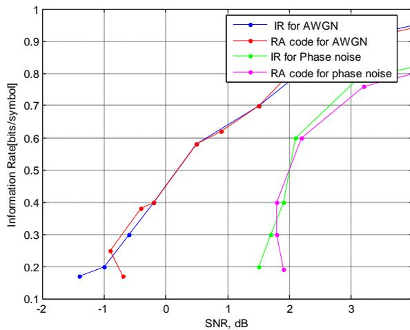
Fig .6. Code rate compared with information rate for a channel with a phase noise with  $\sigma_{\Delta} = 20$  degrees
