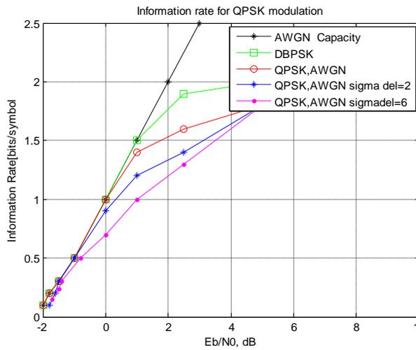
Fig.5. Information rate of QPSK modulation compared with DBPSK modulation.
