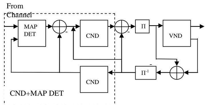
Fig. 1. Iterative receiver for a nonsystematic RA code
