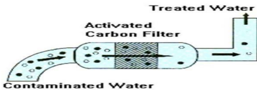
Fig. 7 Typical Activated Carbon Plant
