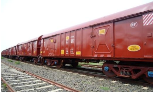
BCNHL WAGON (MICROALLOYED STEEL) WITH SINGLE SLIDING DOOR
