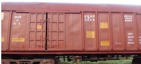
BCNHL WAGON (MICROALLOYED STEEL) WITH TWO PART SLIDING DOOR
