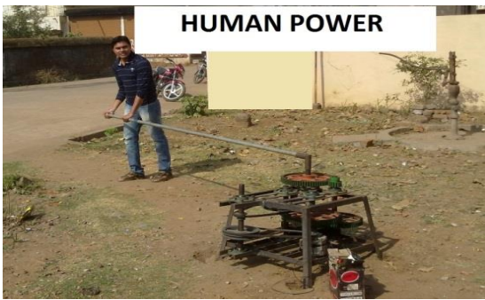
Figure 3: Human muscle power operating to gear reduction system
