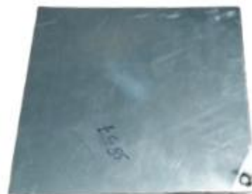
Figure 1 Aluminium 6061 alloy Specimen for Dimensions It is 200 mm long, 200 mm wide, and 10 mm thick
