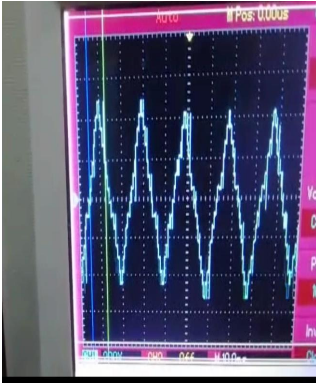
Fig(4.13):Output 15 level Sinusoidal waveform
