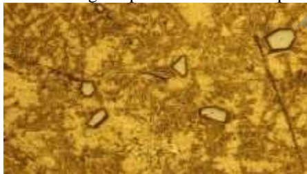
(a) 1.5% glass reinforcement (400X)
