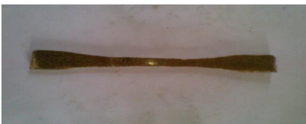
Figure 6: Fabricated and prepared sample as per ASTM for tensile test
