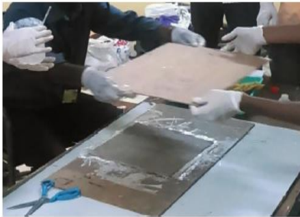
Figure 4: Sample preparation by wet hand layup process
