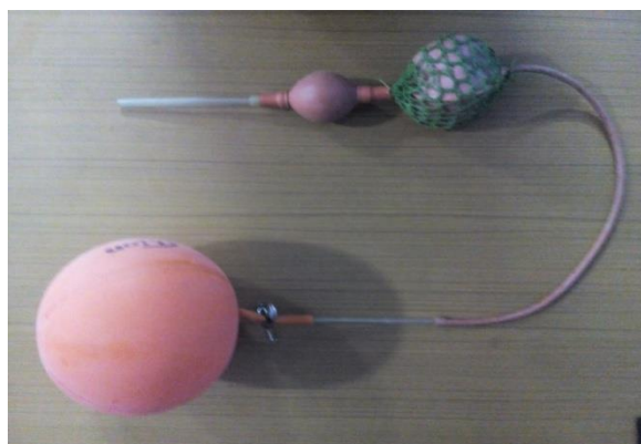
Fig 9, Gas products sample collection bladder.
