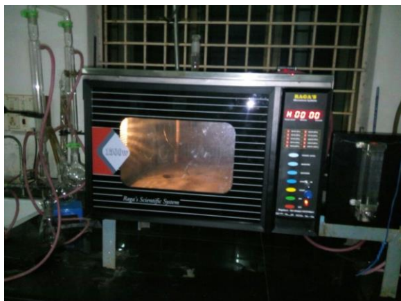
Fig 8, Microwave pyrolysis reactor system.
