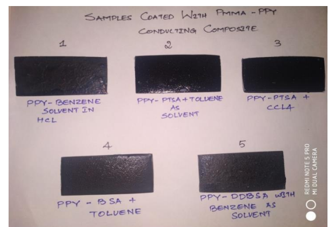
Figure 3: Samples coated with PMMA-PPY.
