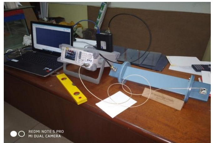
Figure 8: Actual electromagnetic shielding experimental setup.
