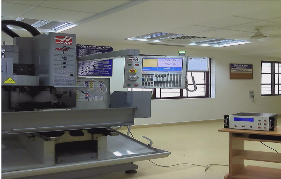
Fig.1. Experimental setup – Syscon tool dynamometer connected with HASS Vertical Machining Centre
