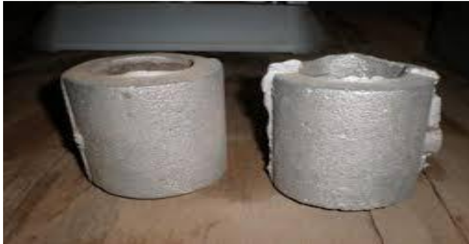
Figure 2.1 Cast test bars of Al-4Si and Al-7Si
