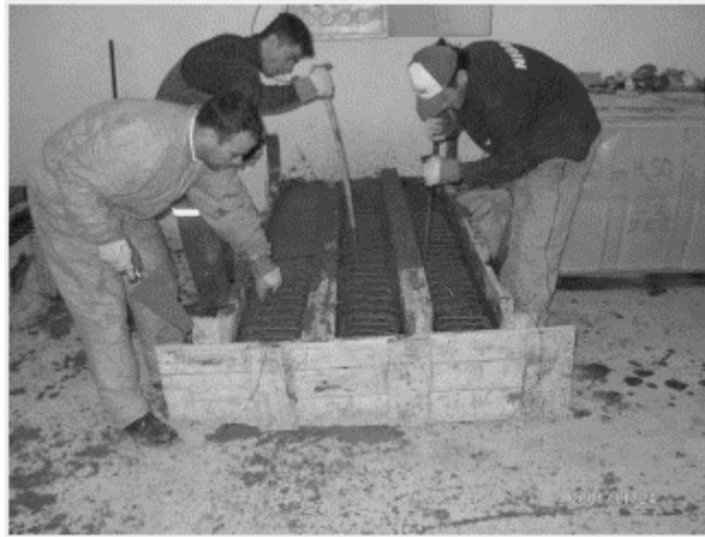
Fig. 7 Concreting of the SFRC beams.
