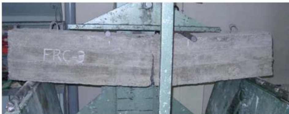
Fig. 8 One of the four-point loading beam-loading experiments
