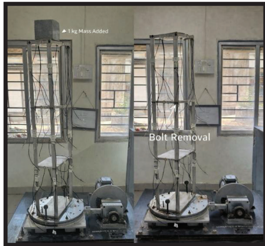
Figure 4: Damage conditions: (a) Bolt removal (b) Mass addition.
