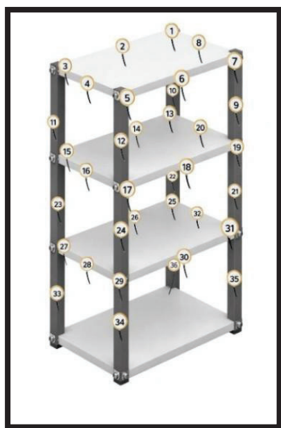
Figure 2: Placement of PZT sensors.
