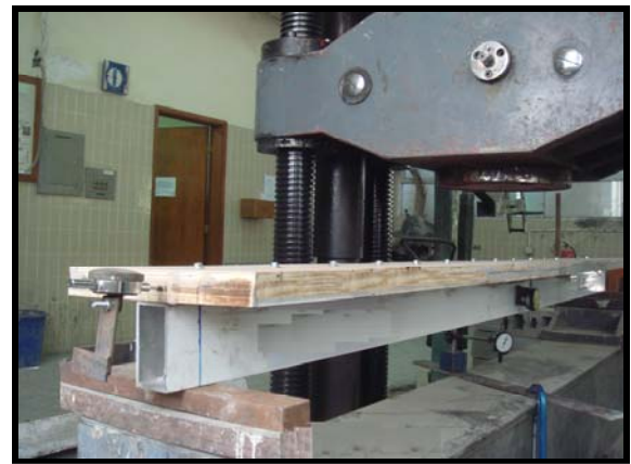
PLATE 1 COMPOSITE BEAM SPECIMENS TEST SETUP
