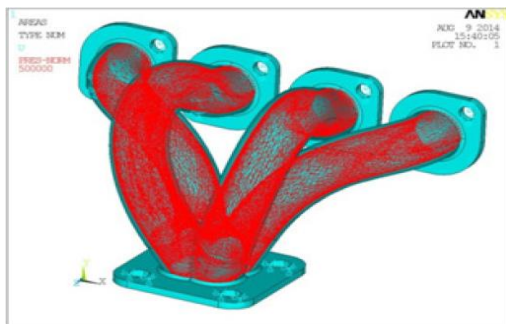
Fig. 10: Manifold–Boundary conditions for Harmonic analysis
