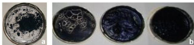
Fig. 2. (a) Pure PANI. (b) PANI doped with different concentrations of m -cresol (5 ml, 10 ml, and 15 ml).
