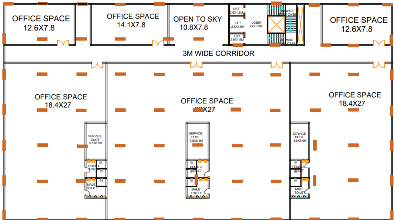
Fig. 2. Column layout superimposed on the building plan.
