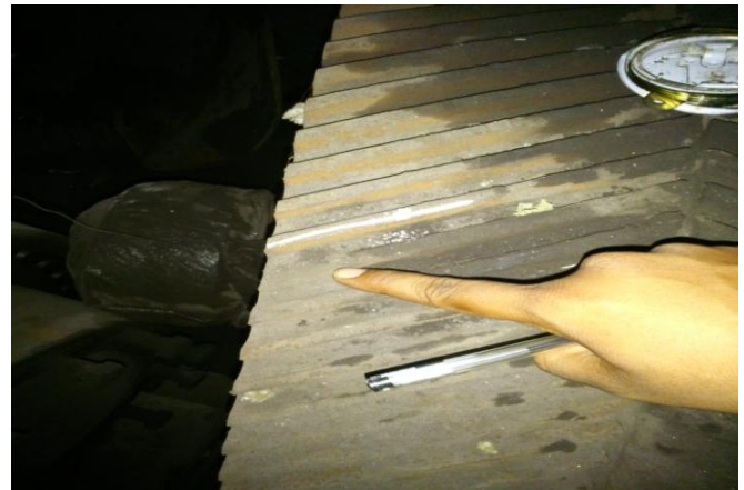
Figure 1. Location of failure of gear tooth
