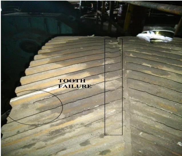
Figure 2. Location of failure of herringbone gear
