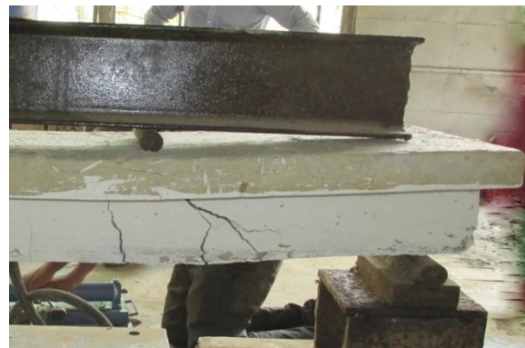
Fig 7 Shear failure of control beam
