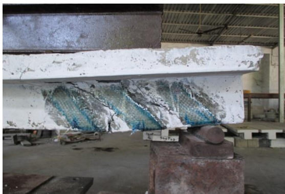
Fig 10 Shear failure in SB4
